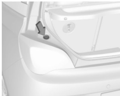
Fit light assembly with the retaining pins into the recesses of
