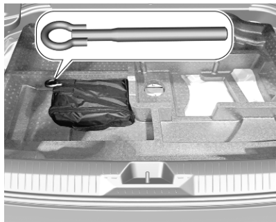
The towing eye is located in a bag. Tyre repair kit ↗ 224.
