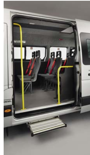
The wide-opening sliding side door and kick-out standard step ensure easy passenger access. LED lights are fitted to all entrances and exits.
