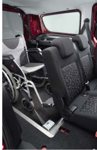
Lowered floor for wheelchair position.
