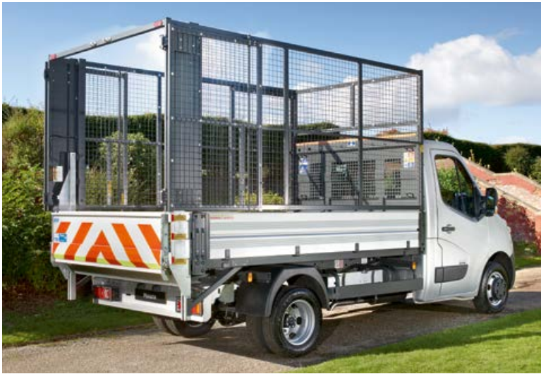
Cage option with 270° opening/lockable rear doors is also available. The 500kg tail lift (illustrated), is also optional.
