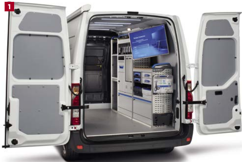
1. Workshop van. L2 H2 Movano fitted with a combination of workshop bench and racking systems.
