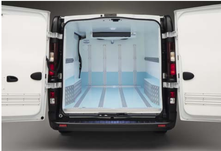
CFC-free, high density lightweight foam insulation panels are fully bonded into the vehicle load area.
