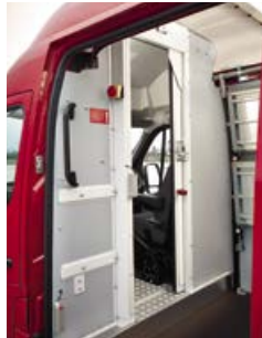
Access to the load area from the cab is through a sliding door.
