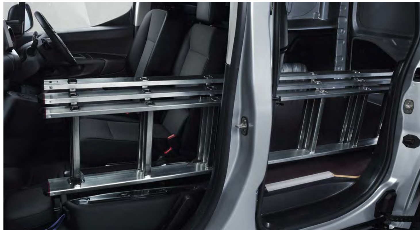
Load-through hatch within bulkhead.
