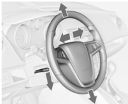
Unlock the lever, adjust the steering
