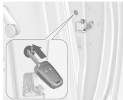
Insert key into the opening above the lock on inside of the door and operate the lock by pressing until it clicks. Then close the door. The procedure must be carried out for each door. The driver's door can also be locked from the outside with the key. The fuel filler flap and the tailgate cannot be locked.
