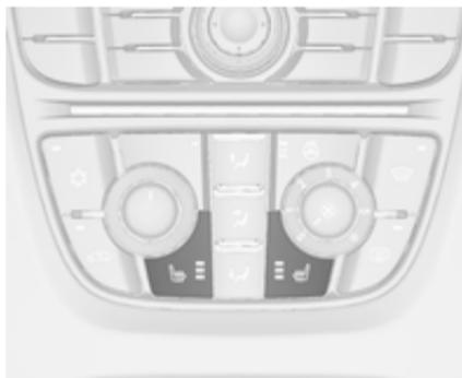
Adjust heating to the desired setting by pressing the
