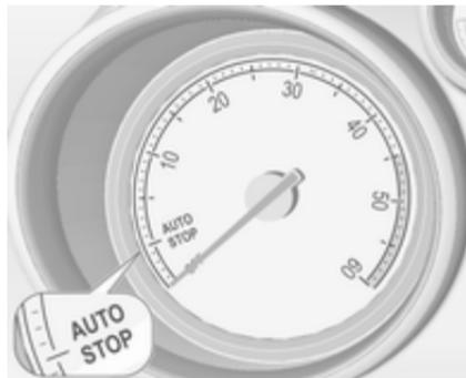
If the vehicle is at a low speed or at a standstill and certain conditions are fulfilled, activate an Autostop as follows:
