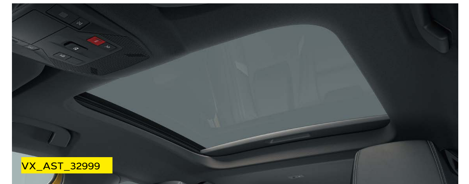
Electrically operated slide/tilt glass sunroof with blind.
