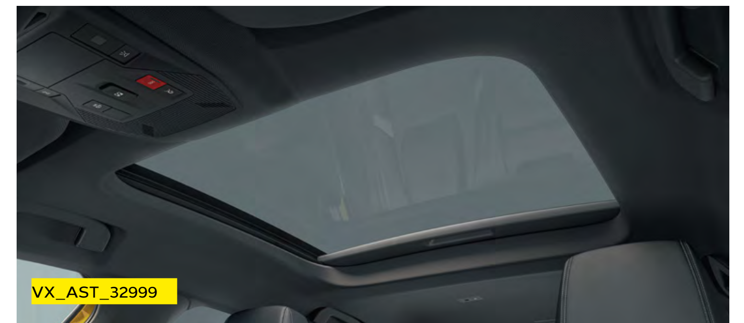
Electrically operated slide/tilt glass sunroof with blind.
