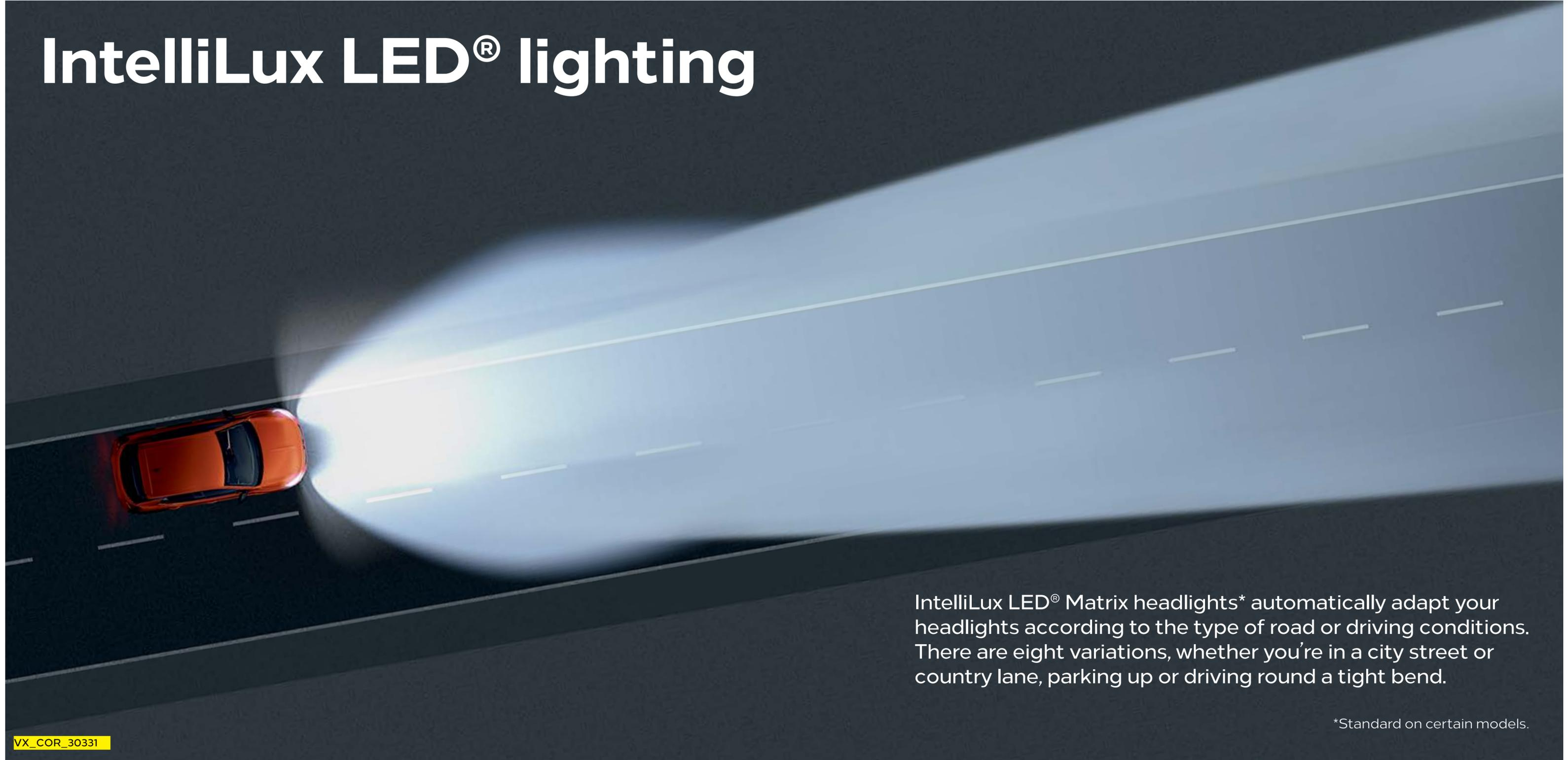
IntelliLux LED<sup>®</sup> Matrix headlights\* automatically adapt your headlights according to the type of road or driving conditions. There are eight variations, whether you're in a city street or country lane, parking up or driving round a tight bend.
