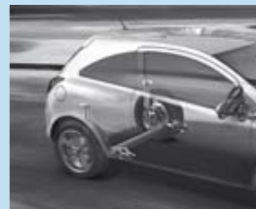
Compound crank rear suspension.
