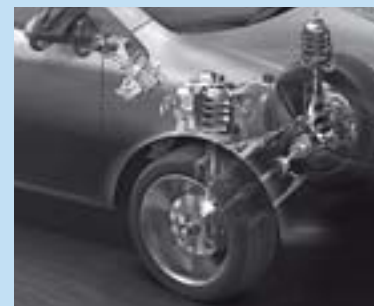
MacPherson strut front suspension.
