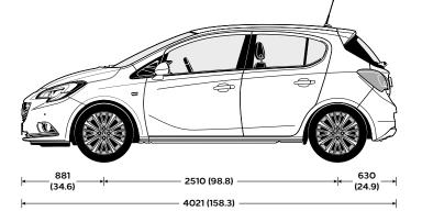
All measurements are in mm (inches) unless stated otherwise. \*Behind front seats. \*\*Measured using the ECIE method.
