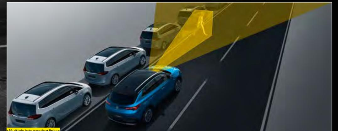
**Automatic emergency braking\***: No trouble ahead with automatic emergency braking. In busy traffic, it warns you if you approach a vehicle too fast, and automatically brakes for you as a fail-safe.
