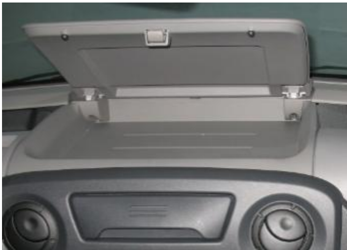
Upper shelf with lid open (Dimension appr. 290 x 390 x 50mm)
