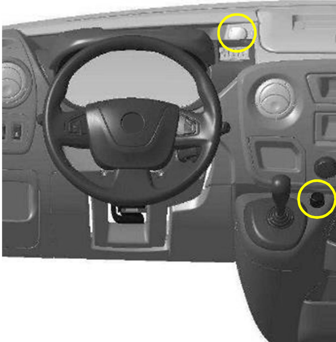
Location of accessory sockets on the dashboard
