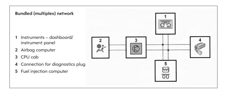
The Vivaro multiplex network enables the 4 computers (CPU cab, fuel injection, airbag and instrument panel) to exchange data.
