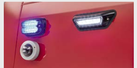
Rear Lighting and CCTV.
