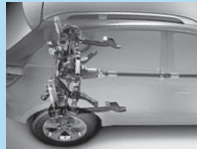
Rear suspension includes automatic self-levelling on 2.0CDTi 16v models.
