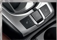
Heated front seats. On all models, heating elements in the seat backs and cushions enable the front seats to reach a comfortable temperature in a very short time. There are three separate heat settings.
