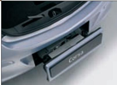
◀▲▶ Most of the time Flex-Fix® stays hidden behind the rear number plate, but when the need arises, you simply extend it, attach the extra rear lights, fix your bikes to the carrier and off you go. An acoustic warning sounds when the carrier is extended and reverse gear is engaged.
