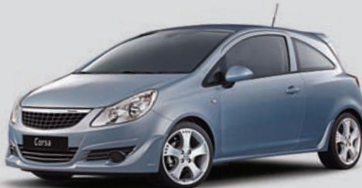
▲ Irmscher Styling Pack\*. Treat your Corsa to the Irmscher Styling Pack which consists of body colour front lower spoiler, side sills, rear hood spoiler and rear bumper sports insert. Vehicle illustrated also features cross hatch grille with aluminium upper and laser-etched 'Irmscher' logo and 17-inch Sport Star alloy wheels.
