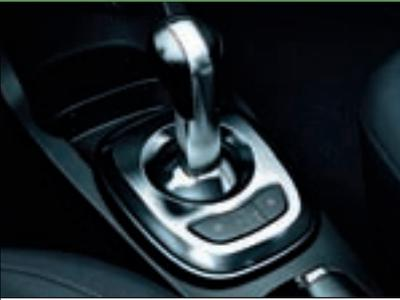
◀ **Easytronic.** Choose Corsa's optional Easytronic transmission and you'll get a five-speed manual gearbox with a fully automatic mode. In manual mode, you simply push the lever forward or back to shift gears up or down and by nudging the lever to the side you switch to fully automatic mode. There's no clutch pedal so you can drive it on an automatic-only driving licence.
