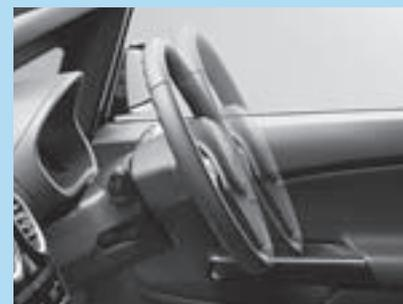
Steering column adjustable for reach and rake.
