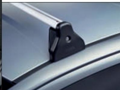
◀ **Base carrier.** The Vauxhall roof rack system begins with this base carrier. It comprises of two T-track bars which support a wide range of attachments. Each carrier is supplied with locks for security.
