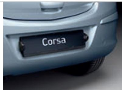
▲ **Rear parking distance sensors.** Helping reduce the risk of bumps and scrapes, this two-sensor, retailer-fit system beeps as you reverse close to an obstruction, changing to a continuous tone when the object is approximately 300mm away.
