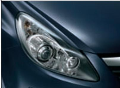
**▼▶ Halogen AFL.** Another feature you don't expect on a car like Corsa, optional Halogen Adaptive Forward Lighting moves the headlight beams up to 15 degrees left or right of the straight ahead position when you turn the steering wheel, helping improve your vision of the approaching bend.
