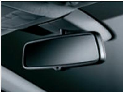
**Rain and light sensors.** Automatic lighting control can switch the car's lights on when it gets dark. Other sensors can switch the wipers on and even dim the rear-view mirror – all automatically. These features are standard on Design and optional as the Sight and Light Pack on SXi and SRi.
