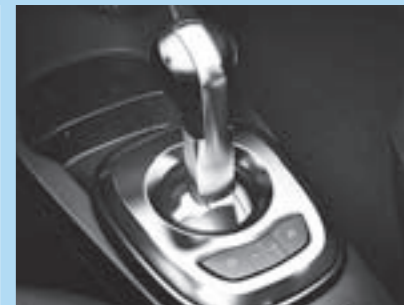
Five-speed Easytronic transmission.
