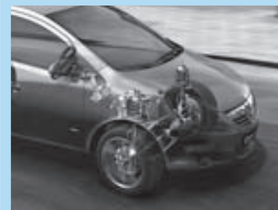
MacPherson strut front suspension.
