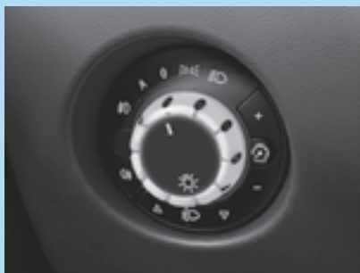
Automatic Lighting Control.
