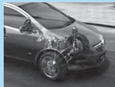
MacPherson strut front suspension.
