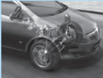
MacPherson strut front suspension.
