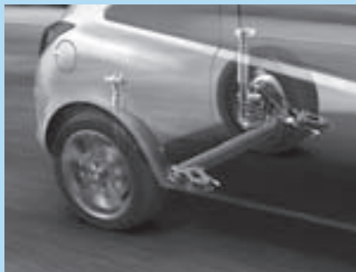
Compound crank rear suspension.
