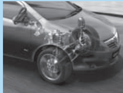
MacPherson strut front suspension.
