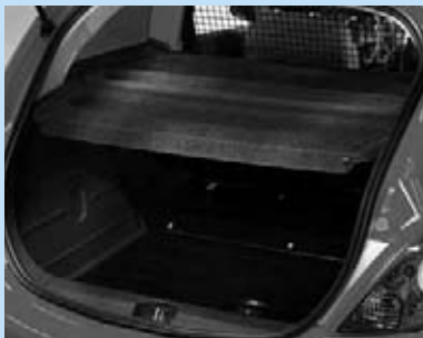
Load compartment cover (four-piece) and upper load restraint mesh.
