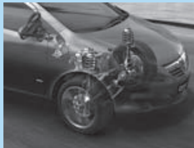
MacPherson strut front suspension.
