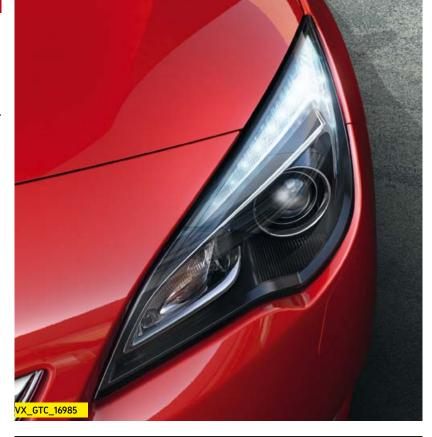
Intelligent Light Ranging (ILR). Available as part of the Driving Assistance Pack when AFL is also specified, ILR extends the range of both headlights up to about 350 metres at speeds over 30mph. ILR also automatically adjusts the spread to avoid dazzling oncoming drivers. And if you're approaching an upward gradient, it'll even raise the beam to give you a better view of the road.
