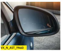
side Blind Spot Alert. Available as part of the optional Perimeter Protection Pack on Sport and SRi models, this ultrasonic-based system helps prevent a potential collision with a vehicle in the neighbouring lane by continuously screening the blind spots on both sides of the car and provides a visible warning if the indicator is set to change to a lane where another car is detected.
