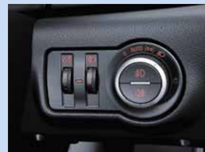
Automatic lighting control.
