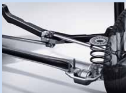
Watt's link improves handling and ride comfort.
