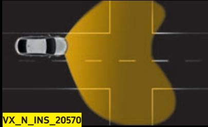
**Pedestrian area light.** Illuminates potential hazards with a wider spread of light – an extra eight degrees left and right (up to 20mph).
