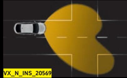
**Town light.** Spreads the beam of light wider and lower. Activated by vehicle speed together with street lighting (20-35mph).
