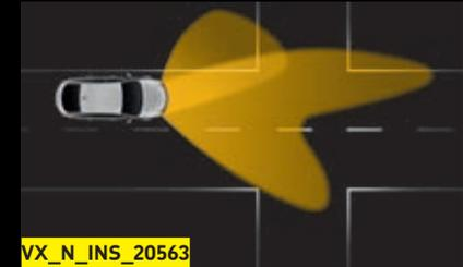
**Static cornering light.** Spreads light 90 degrees to the left or right to help you see better around corners (up to 25mph, also when reversing).
