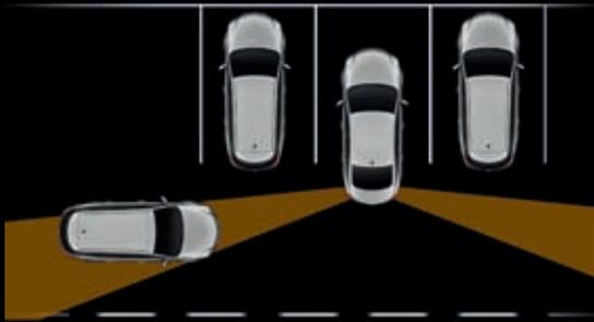
**Rear cross traffic alert.** As you reverse the car in a tricky parking situation this system detects vehicles approaching from the rear and side of your Insignia. The car's speakers then emit an audible warning signal on the relevant side of the car while an icon appears on one side of the centre console display.
