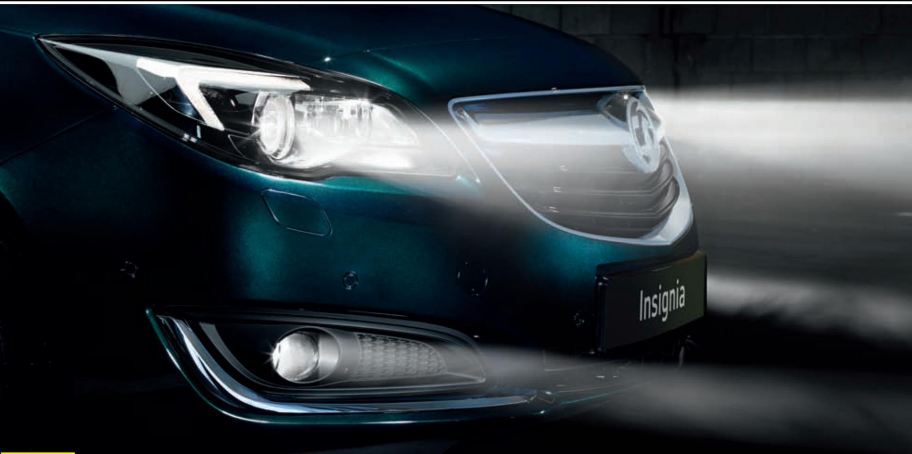
The Insignia can be equipped with the very latest bi-xenon Adaptive Forward Lighting Plus (AFL+) headlight system as an option. This uses a front-mounted camera, rain sensor and steering angle input to improve visibility and safety by automatically adjusting the strength of your headlights to suit different speeds, manoeuvres, weather conditions and traffic situations.
