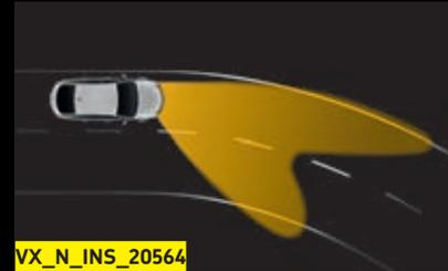
**Dynamic curve light.** Activated by steering angle and speed, the headlights swivel up to 15 degrees into the bend (any speed).
