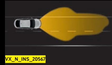
**Motorway light.** 140-metre range, higher and brighter than normal low beam, without dazzle (over 60mph).
