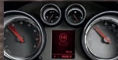
New Insignia's innovative Traffic Sign Memory System recognises speed limit and no overtaking road signs, presenting them on the main display. If you select the speed limit function on the multi-function trip menu, the scanned speed limit is shown permanently until the next sign is recorded. If nothing is recognised, a simple dash will be displayed. Push the speed limit button on the steering wheel and the limit is displayed for just a few seconds.
