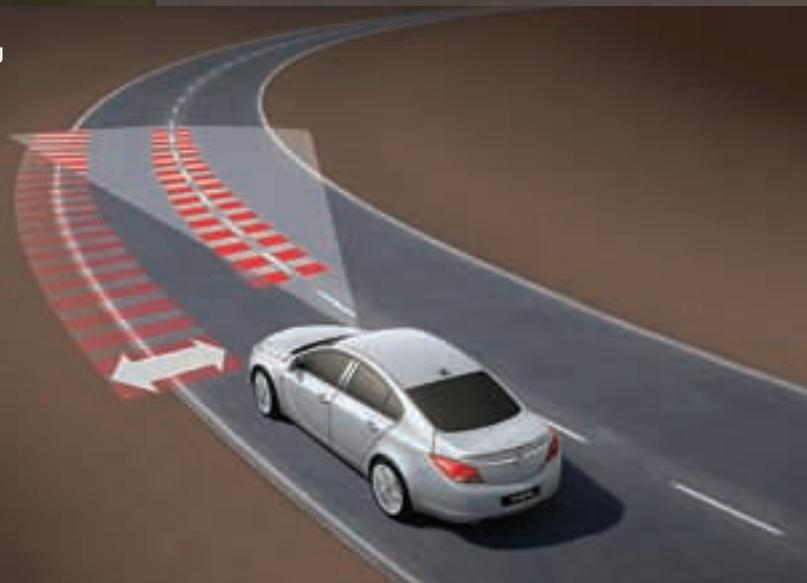
The Lane Departure Warning uses the Front Camera System to recognise lane marking lines and emits an audible warning if the vehicle leaves its lane unintentionally (ie. without you indicating), preventing potential accidents and reminding you of inattention or tiredness. Both systems can be deactivated via the facia switch.
