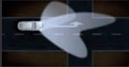
**Static cornering light (up to 25 mph, also when reversing).**
