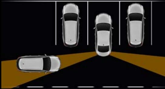
**Rear cross traffic alert.** As you reverse the car in a tricky parking situation this system detects vehicles approaching from the rear and side of your New Insignia. The car's speakers then emit an audible warning signal on the relevant side of the car while an icon appears on one side of the centre console display.
