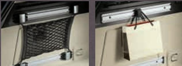
Comprising four side rails with sliding side rail hooks, plus a specially devised 3D storage net and side net pocket, the optional FlexOrganiser® system provides a versatile way to manage the new Insignia Sports Tourer load area. A range of FlexOrganiser® accessories is also available including: storage box, adjustable fixing straps and additional side rail hooks.
