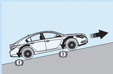
Maintains the brake pressure for a short period after the brake pedal has been released when pulling away on a steep gradient; this helps prevent the vehicle from rolling back. The pressure is released as soon as the driver presses the accelerator and the car begins to move forward.
