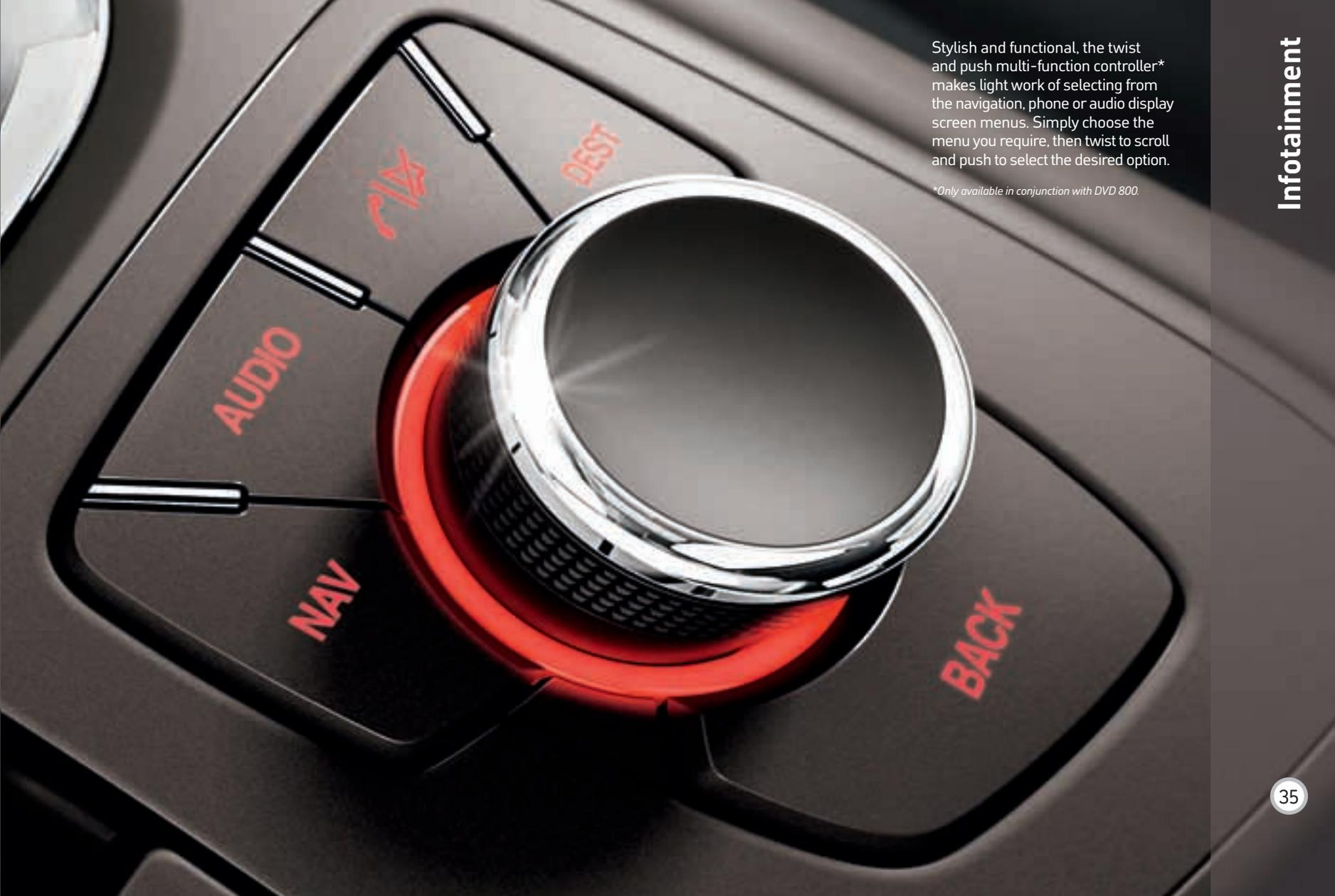
Stylish and functional, the twist and push multi-function controller\* makes light work of selecting from the navigation, phone or audio display screen menus. Simply choose the menu you require, then twist to scroll and push to select the desired option.
