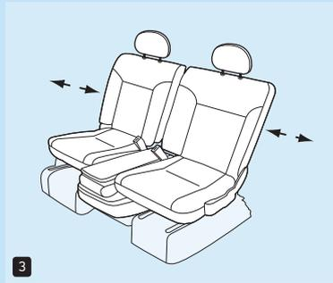
**4** Each rear seat can be individually slid backwards 70mm to provide extra legroom. And each backrest can be reclined a further six degrees (to 29 degrees) to give a truly relaxing travelling environment.
