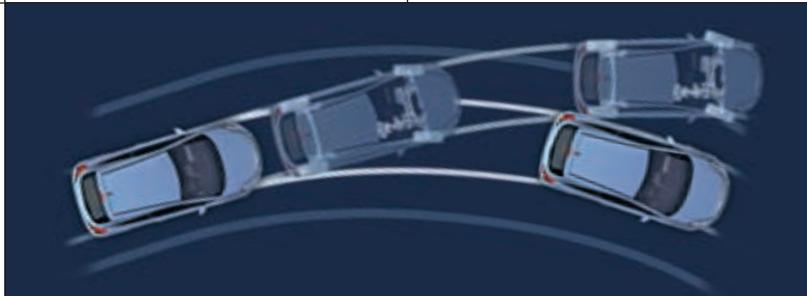
▶ **ESP and Traction Control\*.** Electronic Stability Programme (ESP) helps you maintain control during adverse or emergency conditions. If the car begins to slide, ESP gently applies corrective braking to the appropriate road wheel to help you regain control. Traction Control (TC) helps prevent wheelspin during acceleration. Further explanation can be found in the Technical data section on page 49.
