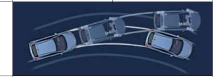
ABS. Meriva's Anti-lock Braking System (ABS) with Electronic Brakeforce Distribution (EBD) and Emergency Brake Assist (EBA) can reduce emergency stopping distances, particularly on slippery roads. It prevents the wheels from locking up and allows drivers to retain steering control.
