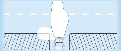
Employs an additional reflector which projects a beam of light approximately 90° to the direction of travel. This 'wide angle' effect provides enhanced illumination of side roads and junctions. The system is speed dependent.
