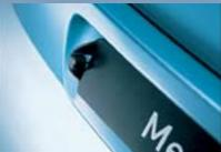
Rear parking sensors. This invaluable parking aid is mounted within the Meriva rear number plate area. Activated automatically when reverse gear is selected, it beeps as you approach an obstruction rising to a continuous tone when it's approximately 300mm away.
