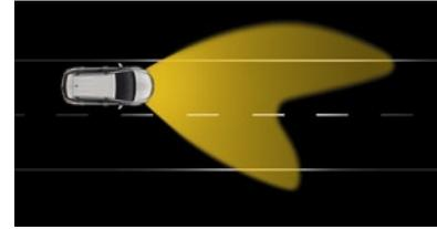
**Country road light (35–70mph).** Wider spread and brighter light than normal low beam. 70 metre range without dazzle.
