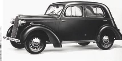
1937 – The Vauxhall 10' H-type, the first British car to have integral construction.
