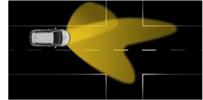
**Static cornering light (up to 25mph, also when reversing).** Throws light 90 degrees left or right for enhanced lateral vision.
