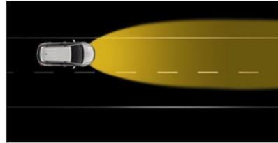
**High beam assist (over 25mph).** Automatically switches from high to low beam as it detects oncoming or preceding vehicles.
