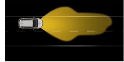
**Motorway light (over 60mph).** 140 metre range, higher and brighter than normal low beam, without dazzle.
