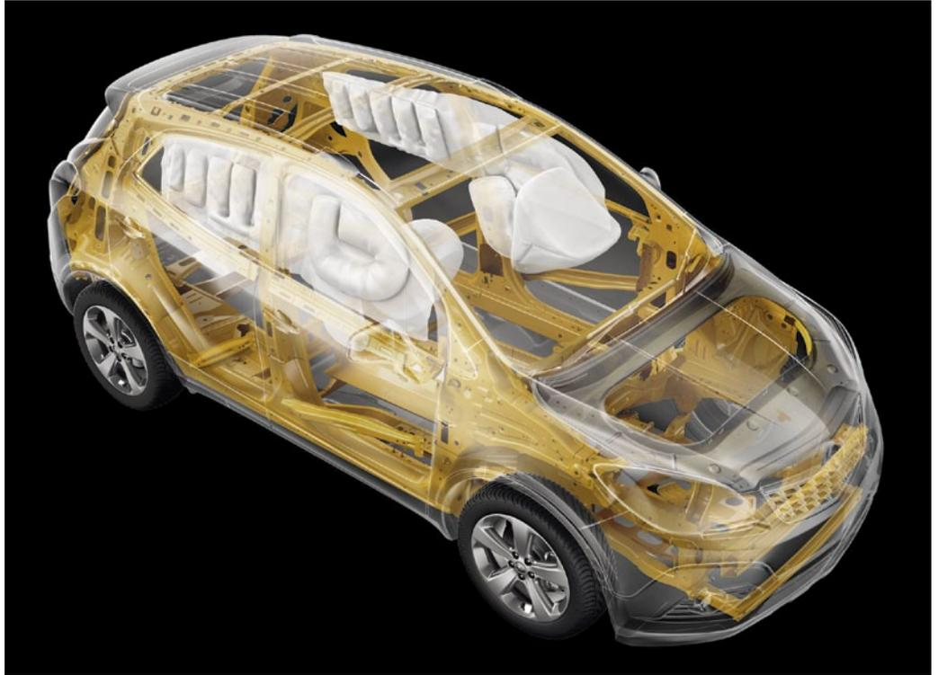
**The Mokka's passive safety systems are uncompromising and comprehensive.** It's difficult to imagine how you could be better protected inside your Mokka. You are surrounded by a high-strength steel rigid passenger cell as well as front, side and full-length curtain airbags. On the outside, pedestrians are protected by bumpers that use low-density foam, designed to reduce the risk of leg injuries should the unthinkable happen.
