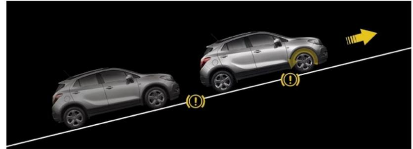
**Hill Start Assist (HSA).** HSA will stop you rolling back unintentionally on steep hills, by automatically releasing the brake at just the right moment when pulling away on a gradient.
