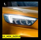
1. Optional Adaptive Forward Lighting LED headlights light the road better as you turn into bends, and also mean you don't have to switch manually between high and low beam.
