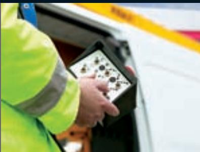
◀ ▶ Vivaro conversions feature a remote boom control wanderlead and are designed to have minimum rear overhang and intrusion into the load area.
