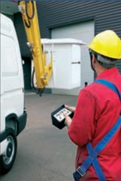
◀ Standard five-metre boom control 'wanderlead' allows easy operator training, with the ability to lift lightweight equipment without an operative in the bucket (eg. to test aerial reception) and the capability to get an operator down in an emergency situation.
