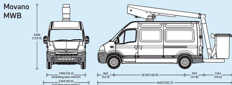
Measurements are shown in millimetres (inches). All heights are shown unladen. Conversion dimensions are estimated and will vary upon specific conversion.
