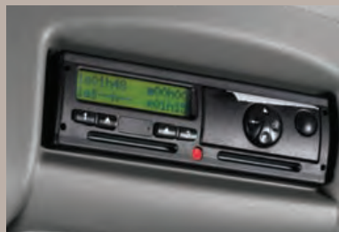
Digital tachograph Computes driving and rest time, enabling fleet management data to be analysed (standard on 4500 HD models).
