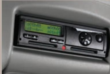
**Digital tachograph.** Computes driving and rest time, enabling fleet management data to be analysed.
