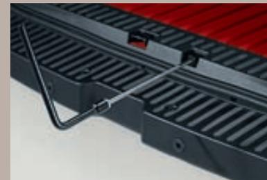
**Under-floor spare wheel.** Unlike spare wheels that are accessed or stored in the load area, Movano's under-floor stowage system means that you don't need to unload the van to get to the spare. And, acting as an additional security measure, the spare wheel can only be winched when the rear door has been unlocked and opened.
