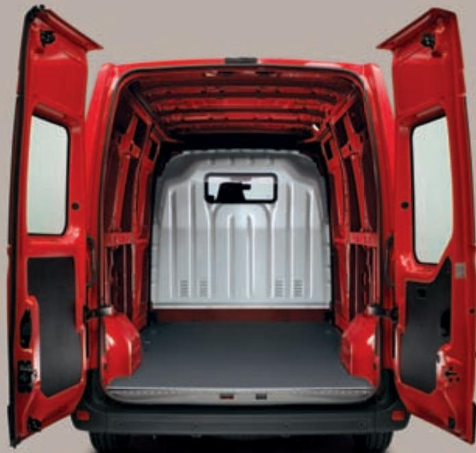
*Resin-coated plywood floor, window for bulkhead and glazed rear doors are optional at extra cost.*
