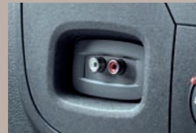
**Auxiliary-in socket.** Lets you connect most MP3 player devices fitted with a headphone output.
