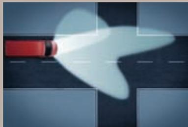
**Static cornering lights.** Depending on the steering angle and vehicle speed when cornering, an additional light illuminates the corner of the road when turning. Static cornering lights are part of the optional Lighting Pack.
