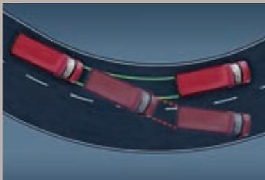
**ESP with TCS.** Standard on all rear-wheel drive models and optional at extra cost on front-wheel drive, ESP reduces throttle response and varies the braking force to each of the wheels when a driving imbalance is detected, keeping the vehicle moving in the right direction. TCS senses a lack of traction during acceleration and reacts to ensure maximum contact between the road surface and the tyres. Page 51 has all the technical detail.
