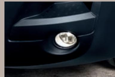
**Front fog lights.** Improved forward vision and reduced glare in foggy weather conditions.
