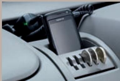
**12-volt accessory cab sockets.** Recognising the increasing need to operate electrical devices, Movano features two 12-volt sockets in the cab and a third in the load area is available as part of the Office Pack.
