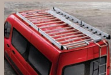
**Walkway for roof rack tray.** Made from lightweight but sturdy perforated aluminium and for use with the roof rack tray, the walkway enhances access to the roof.
