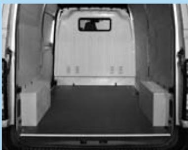
Full-height plywood load lining panels and wheel arch protection.
