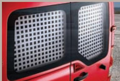
**Rear window protection grilles.** Constructed from 1mm thick epoxy coated steel, the rear window protection grilles help avoid theft while retaining rearward visibility.
