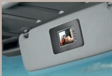
**Rear-view camera.** The 3.5-inch LCD monitor screen, mounted in the driver's sunvisor, is activated by selecting reverse gear, providing a view of the area behind the vehicle.
