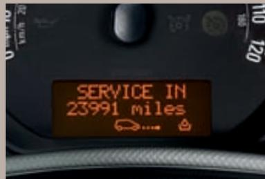
**Trip computer.** Functions: overall distance covered, trip distance, average mpg and speed since last reset, instantaneous fuel used, remaining miles plus service due indicator.
