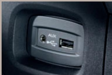
**USB facility.** CD 30 BT units can be specified with a USB facility, allowing drivers to view iPod™ functionality via the audio display.
