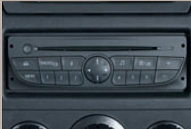
**CD 30 BT.** New Movano drivers can upgrade their audio system with the optional CD 30 BT unit which has the same features as the CD 10, but with Bluetooth® connectivity, a remote monochrome display (illustrated below) and four 20-watt speakers.
