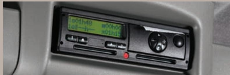
**Digital tachograph.** Easily operated by the driver, the digital tachograph reliably computes driving and rest time, enabling fleet management data to be collected and analysed in a simple and user-friendly manner. It is supplied uncalibrated. This feature is standard on all 4.5 tonne GVW models and optional at extra cost on other models. Please refer to page 38 for further details.
