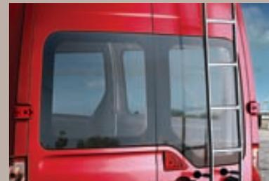
**Steel ladder.** Steel-constructed but with a smart, aluminium-look finish, the rear ladder is firmly affixed to the rear door of the vehicle.
