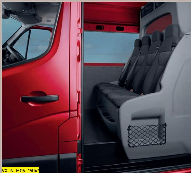
The rear compartment is all the more practical for being only partially trimmed – making it a lot more workmanlike and low maintenance. Despite the rear seats, loadspace volumes remain impressive, up to 9.0cu.m and the windowed bulkhead has been cleverly recessed to maximise load floor length. Finally, with a choice of vehicle lengths, engines and front or rear-wheel drive models, the Doublecab is a natural choice for a multitude of operations.
