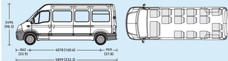
Measurements are shown in millimetres (inches). All heights are shown unladen.
