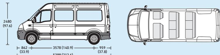
Measurements are shown in millimetres (inches). All heights are shown unladen.
