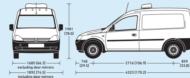
Measurements are shown in millimetres (inches). All heights are shown unladen.
