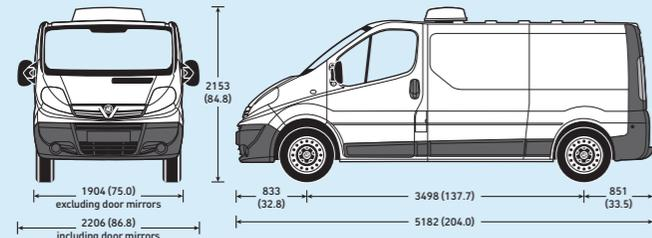
Measurements are shown in millimetres (inches). All heights are shown unladen.
