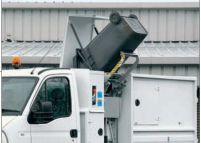
• **The tipping mechanism** features a high performance electro-hydraulic power pack with visible oil level plastic tank and weather protected motor and electrics. The tipping action can be easily operated by one person using hand-held controls on a wander lead, complete with harness and magnetic base, located on the driver's side of the cab. A warning bleeper sounds when the tipper is raised.
