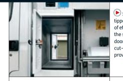
▲ Lockable storage locker provides secure stowage for brushes, gloves and other essential equipment used by the municipal services. The locker is conveniently situated behind the main cab area and can be accessed from either side of the vehicle for maximum ease of use.
