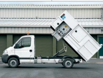
Side bin lift allows rubbish to be tipped into the vehicle with the minimum of effort. Operated by controls situated on the side of the vehicle, above the locker door, the lift features an emergency cut-off switch. Lockable side doors provide an additional means of access.
