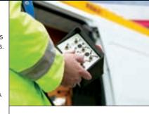
Vivaro conversions feature a remote boom control wanderlead and are designed to have minimum rear overhang and intrusion into the load area.
