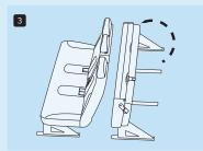
Combi's 'stow and fold' third-row seats (1-3) convert the 9-seat Combi into a six seater with additional luggage space, without having to remove any seats from the vehicle.
