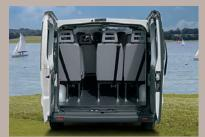
'Quiklok'. Fourth-row seats are mounted on aluminium rails with 'Quiklok' quick-release fittings.
