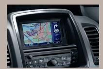
Satellite navigation. Optional TomTombased system features a useful facia mounted/hand-held remote control unit.
