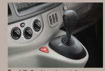
**Tecshift**. Combines the main features and flexibility of automatic transmission with the performance and control of a manual gearbox.
