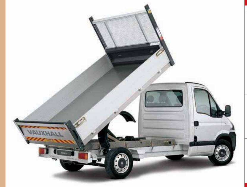
Medium wheelbase chassis cab tipper model
