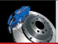
Braking systems. For the driver who wants even more stopping power, VXRacing have developed, with AP Racing, a front braking system using four-pot calipers with larger diameter ventilated discs, high friction brake pads and braided hoses.
