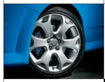
Alloy wheels. The 18-inch sixspoke alloy wheel (left) is standard for Astra VXR, with 225/40 R 18 ultra-low profile tyres. The 19-inch multi-spoke alloys with anthracite inner and 235/35 R 19 tyres (illustrated right) are optional at extra cost.
