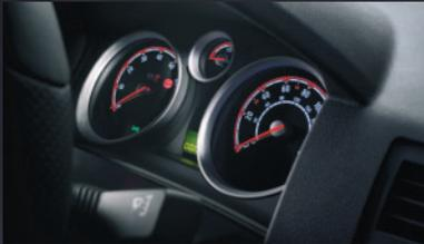
The black sports instruments – with stepper motor speedo and tachometer – feature translucent rings and red highlights. A cool piano black centre console and steering wheel inserts complete the picture.
