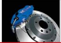
Braking systems. For the driver who wants even more stopping power, VXRacing have developed, with AP Racing, a front braking system using four-pot calipers with larger diameter ventilated discs, high friction brake pads and braided hoses. Specifically designed for the Astra VXR, the kit fits other models.
