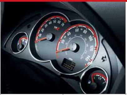
Maximum control. As you'd expect, Meriva VXR comes with something special on the facia and centre console. There's the VXR instrument panel with red speedo and tacho needles, airconditioning and a CD 30 stereo radio/ CD with MP3 capability. Cruise control is standard too.
