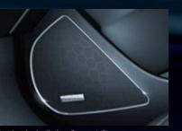
**Insignia Infinity Sound System.** Featuring a 7x45W amplifier and nine premium speakers the system digitises the audio signal so it can be fine tuned with Digital Sound Processing (DSP) for superb all-round sound reproduction under all driving conditions.
