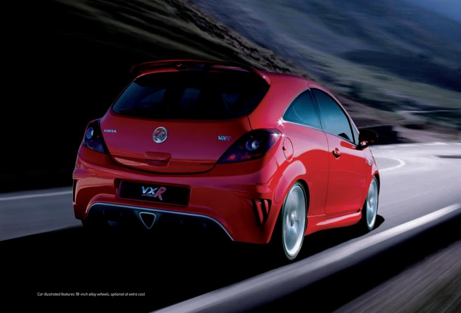
Whichever way you look at it, New Corsa VXR doesn't hang around. The lightweight 1.6 litre turbo puts out 192PS and the software controlled overboost increases maximum torque to 260+Nm for safer overtaking. No worries in the chassis department either. With lowered sports suspension, bigger brakes, switchable Electronic Stability Programme (ESP) with traction control and ABS with straight line stability control and cornering brake control – it's all designed for rapid, safe progress.
