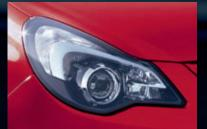
Adaptive Forward Lighting (AFL). Optional on New Corsa VXR, the lighting system swivels the beams up to 15 degrees for improved vision as you turn a corner. On Insignia VXR, the standard Intelligent AFL bi-xenon headlights automatically adjust to suit the driving conditions.
