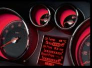
VXR instruments. Insignia VXR takes care of driver information via a wellappointed cluster of red accented instruments, with digital graphic display of oil temperature, oil pressure and boost pressure figures.
