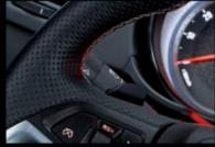
Automatic transmission with paddleshift. Insignia VXR is now available with a six-speed automatic transmission complete with steering wheel mounted paddle-shift for fingertip sequential gear changes.
