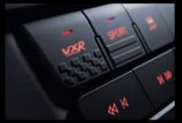
**VXR button.** Hit the VXR button and the Insignia VXR tightens the suspension, sharpens the throttle response and makes the steering more direct.
