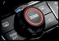
**Electronic Climate Control (ECC).** The dual-zone climate control system allows variable side-to-side temperature settings to be selected.
