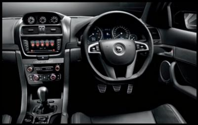
**Performance facia.** The New VXR8 GTS steering wheel means business – leathercovered and flat-bottomed with perforated grip zones and remote audio controls. The steering column is reach and rake adjustable too. Other features include a stateof-the-art infotainment system featuring CD player with USB connection and auxiliary-in socket, integrated iPod<sup>™</sup> support and Bluetooth<sup>®</sup> connectivity.
