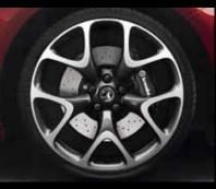
Optional at extra cost as part of the VXR Aero Pack, 20-inch five-Y-spoke forged bi-colour alloy wheels with 245/35 R 20 ultra-low profile tyres.
