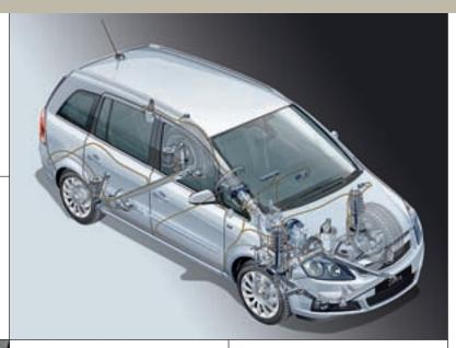
**ESP-plus.** Especially useful on wet roundabouts and greasy roads or whenever a slippery surface catches you out, Electronic Stability Programmeplus (ESP-plus), senses if the car starts to slide on a bend and applies corrective braking to the appropriate wheels to help you regain control. For further information please see page 51.
