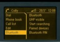
Mobile phone system with Bluetooth®\*. With the optional mobile phone system, your phone interfaces with the audio unit, for operation via the steering wheel controls and facia display. Bluetooth® wireless technology with voice activation is included. See page 45 for more detailed information.
